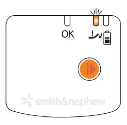
The orange light will flash like this if the pump cannot reach the proper vacuum level.
