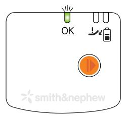
While the PICO pump is working correctly a green light located at the top of the device will flash continuously.
