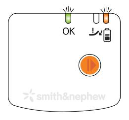
The green light and the orange light above the battery will flash together when the batteries need changing.
